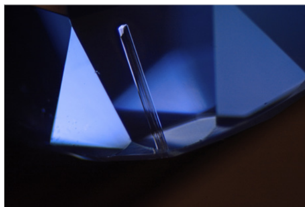
Figure 4 Prismatic green hornblende inclusion (amphibole) in sapphire from Kashmir, India. The inclusion was identified using Raman microspectroscopy. These types of green hornblende needles are a characteristic inclusion in sapphire from India and allow experienced gemologists to determine the origin of the cut sapphire in a piece of jewelry. GEMMASTER with ZEISS Stemi 508; dark-field illumination, magnification: 50x Courtesy of the Swiss Gemological Institute SSEF
