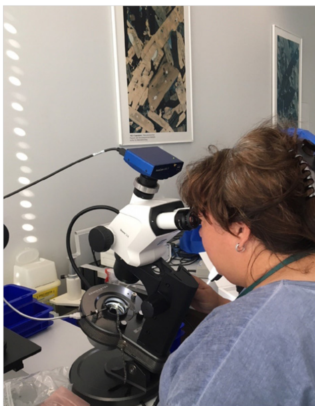
Figure 2 GEMMASTER is an ergonomic, tilted base equipped with focused LED lighting. ZEISS Stemi 508 provides the observation optics and captures the scattered light.
