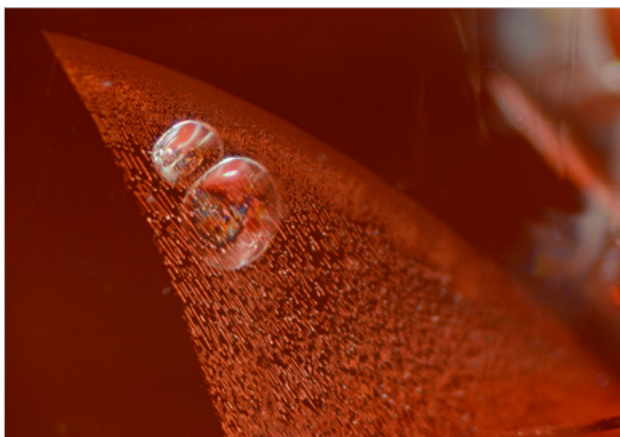
Figure 5 The two round atoll-like explosive fractures coming from a natural healing crack with a number of tube-shaped liquid inclusions prove that the orange sapphire being examined was heated. Adamantine spar (ruby and sapphire) is frequently heated to improve its color and transparency. For this reason, it is important with adamantine spar to always check whether it is untreated or has been heated. This factor significantly impacts the price of the gemstone.
