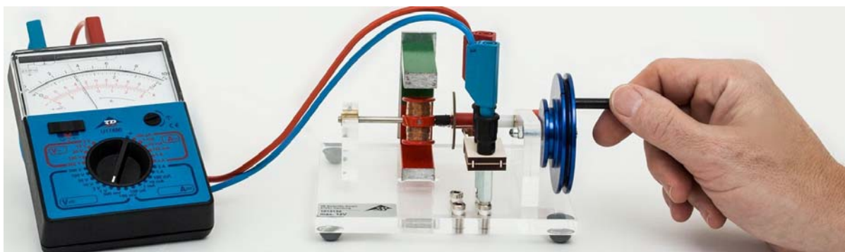
Fig. 3 Operation as a DC motor with ESCOLA 10 multimeter
