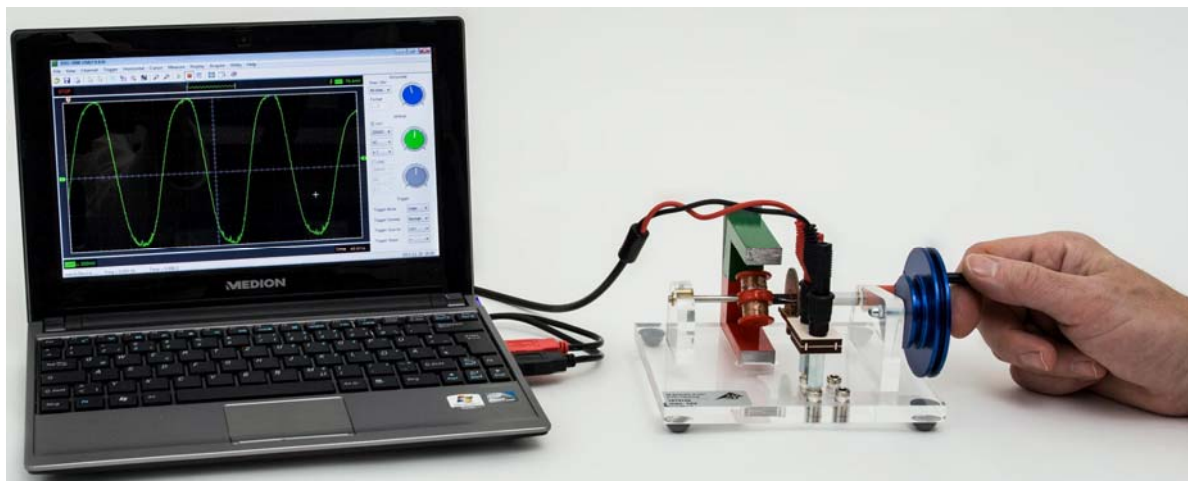
Fig. 5 Operation as an AC generator with a USB oscilloscope
