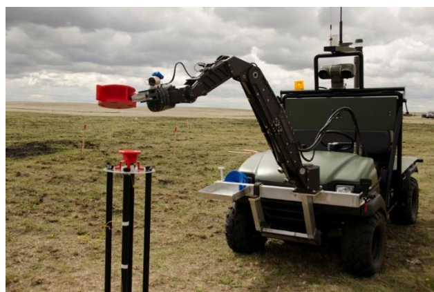
3 – PHOTO: This MATS vehicle, equipped with a robotic arm, handles a highly radioactive material used for a trial at DRDC – Suffield Research Centre . The MATS system allows the operator to stay a safe distance away during manipulation of the source.
